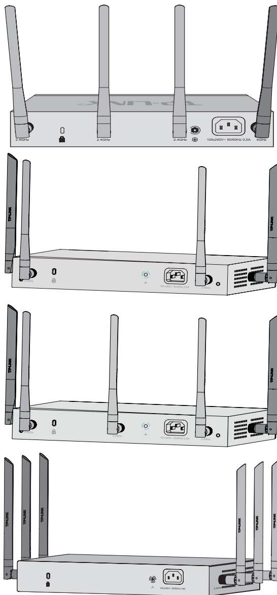
图1-12 TL-WVR900G/TL-WVR1200G/TL-WVR1300G/TL-WVR1750G后面板示意图
